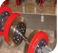
EPROX provides standard pigging, Our pipeline pigging program consist the manufacture of poly foam pigs, decoking pigs, moni-directional pigs fitted with cups (standard scraper or conical) and bi-directional pigs fitted with discs (soft sealing, hard guiding) and custom made pigs starting at size 2" upto 100" for poly foam pigs and size 4" upto 60".
